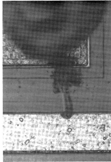
Figure 4-1: Flashover Bondpad - Ground, Damage to the Oxide Layer by HPM (80 kV/m) Component: 7404AN/TTL (Inverter)
